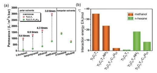
Fig. 6 (a) Comparison of hydrophilic  $Ti_3C_2T_x$  and hydrophobic  $Ti_3C_2T_x-C_{12}H_2$  membrane permeabilities, and (b) interaction energies between membrane and solvent.<sup>53</sup> This figure has been reproduced from ref. 53 with permission from the Wiley Online Library, Copyright 2019.
