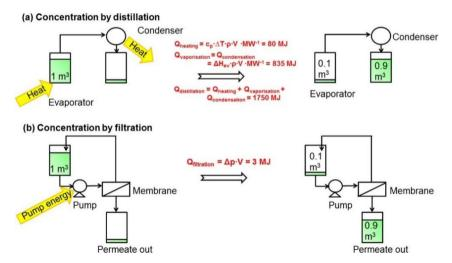
Fig. 3 Comparison of consumed energy by (a) distillation and (b) OSN processes to concentrate 1 m<sup>3</sup> of a dilute solution in methanol by a factor of 10.<sup>1</sup> This figure has been reproduced from ref. 1 with permission from American Chemical Society, Copyright 2014.
