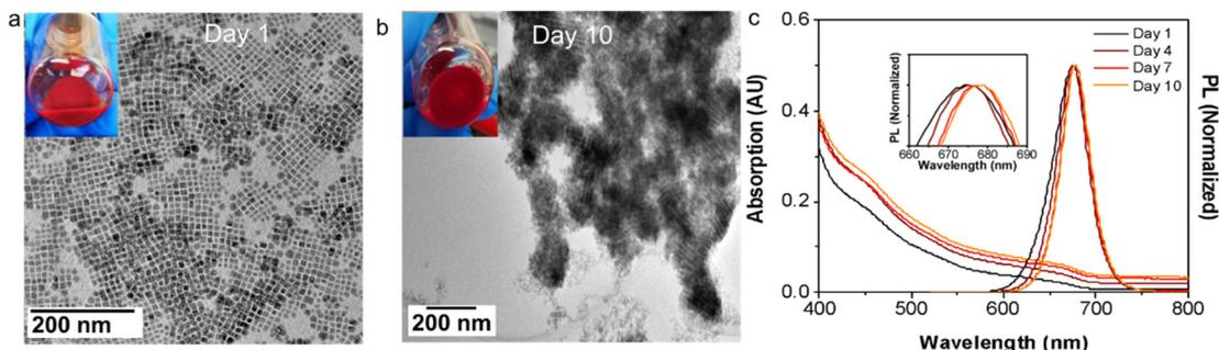
Fig. 5 TEM images and photos for the CsPbI<sub>3</sub> crude solution synthesised with Cs : Pb : I = 1 : 4 : 8 stoichiometry that is (a) as-synthesised, (b) stored for 10 days, and (c) evolution of corresponding UV-vis absorption and PL spectra with time (inset: zoom-in PL spectra showing the redshift of the PL peaks).
