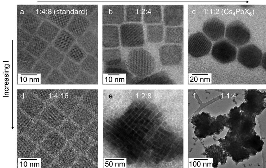
**Fig. 2** TEM images of CsPbI<sub>3</sub> NCs synthesised using HDA-HI at different Cs:Pb:I molar ratios: (a) 1:4:8, (b) 1:2:4, (c) 1:1:2, (d) 1:4:16, (e) 1:2:8, and (f) 1:1:4. All images were taken immediately after synthesis.
