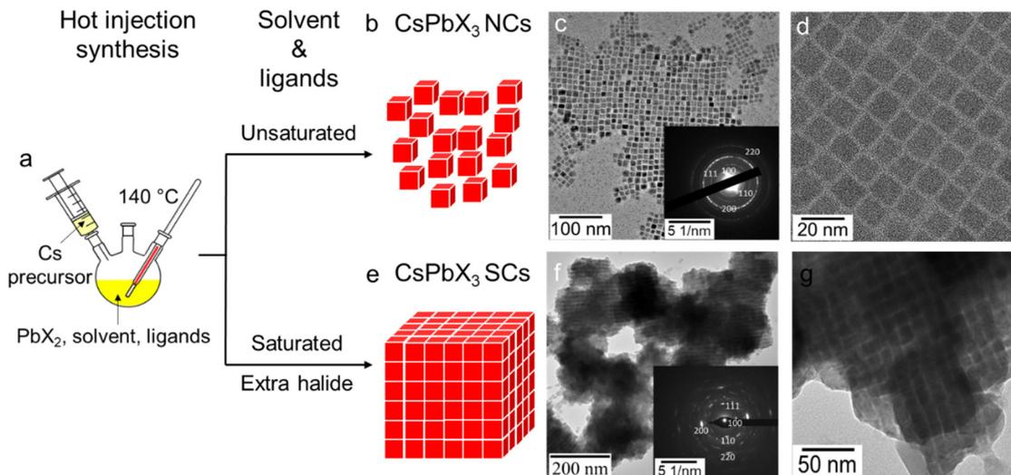
**Fig. 1** (a) Schematic illustration of CsPbX<sub>3</sub> NC and SC syntheses. Structure illustration, low and high magnification TEM images for (b)–(d) CsPbI<sub>3</sub> NCs and (e)–(g) SCs. Insets of (c) and (f) are indexed SADP of NCs and SCs.
