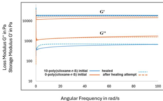
Fig. 11 Storage modulus ( $G'$ ) and loss modulus ( $G''$ ) measurements of 0-poly(siloxane- $r$ -S) (orange) and 10-poly(siloxane- $r$ -S) (blue) initial (solid line) and after healing attempt (dotted line).
