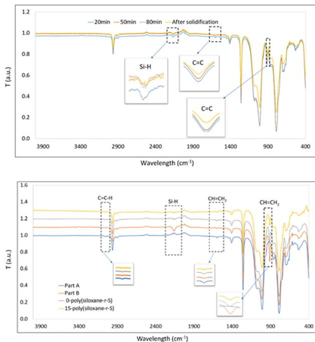
Fig. 4 Top: FT-IR spectra of (a) 10-poly(siloxane- $r$ -S) after reacting with sulfur for 20 min (blue), 50 min (orange), 80 min (grey) and after solidification (yellow), and bottom: part A (blue), part B (orange), and 0-poly(siloxane- $r$ -S) after stirring for 2 h (grey) and 15-poly(siloxane- $r$ -S) after solidification at 180 °C (yellow).
