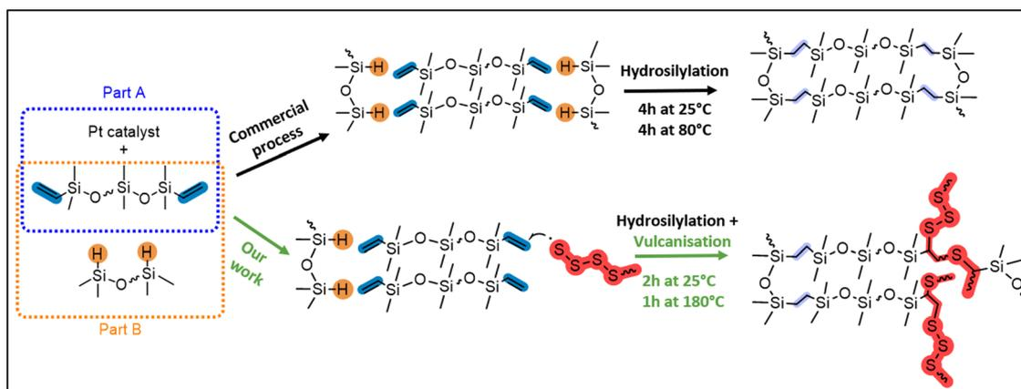
Fig. 2 Commercial synthesis (top route) of polysiloxane from the part A and part B moulding kits and our modified synthesis (bottom route) using S<sub>8</sub> to generate X-poly(siloxane-*r*-S) (X = wt% S) with thermally repairable properties.
