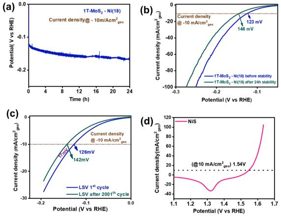
Fig. 6 (a) A 24-h-long durability study (steady state CP test) at a current density of  $-10 \text{ mA cm}^{-2}_{\text{geo}}$ , (b) comparison of the cathodic polarization curves before and after the 24-h stability test. (c) ADS experiment (cyclic stability test) of 1T-MoS<sub>2</sub>-Ni(18) towards the alkaline HER. (d) Backward anodic polarization curve (100% iR corrected) for NiS towards the alkaline OER.
