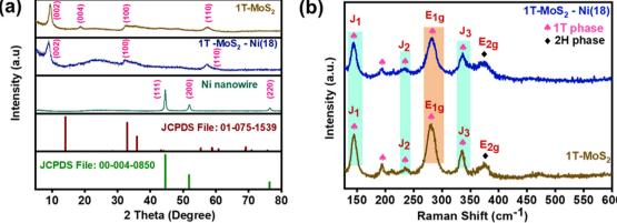
Fig. 2 (a) PXRD patterns of the Ni nanowire, 1T-MoS<sub>2</sub> and 1T-MoS<sub>2</sub>-Ni(18) as compared with the standard patterns of MoS<sub>2</sub> (JCPDS File No. 01-075-1539) and metallic Ni (JCPDS File No. 00-004-0850). (b) Raman spectra of the as-synthesized 1T-MoS<sub>2</sub> and 1T-MoS<sub>2</sub>-Ni(18) composite material.
