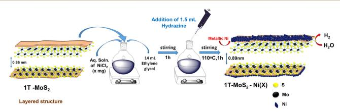
Fig. 1 Schematic representation of the synthetic protocol to prepare the 1T-MoS<sub>2</sub>-Ni(X) composite structure.
