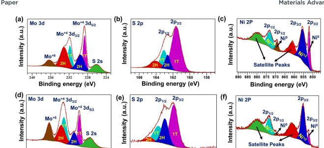
Fig. 4 High-resolution deconvoluted XPS scan of (a) Mo 3d, (b) S 2p for 1T-MoS<sub>2</sub>, (c) Ni 2p for metallic Ni nanowire, (d) Mo 3d, (e) S 2p, and (f) Ni 2p for as-prepared 1T-MoS2-Ni(18) composite material
