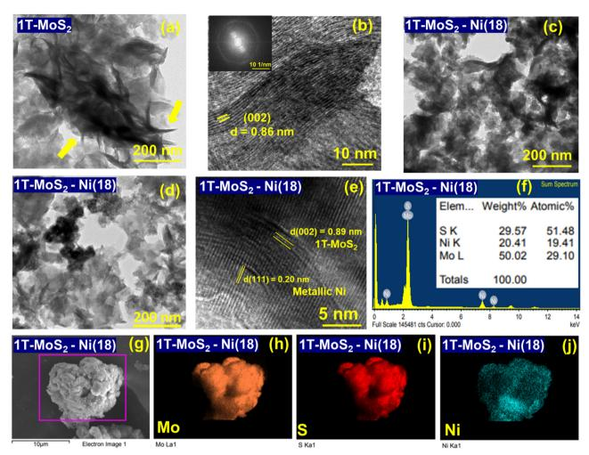
Fig. 3 (a) and (b) TEM and HRTEM images of 1T-MoS<sub>2</sub>, respectively (the FFT patterns of the corresponding HRTEM images are shown in the inset of figure b). (c) and (d) TEM and (e) HRTEM images of the 1T-MoS<sub>2</sub>-Ni(18) composite material, (f) EDS analysis, and (g)-(j) elemental mapping study of as-synthesized 1T-MoS-Ni(18) composite material.
