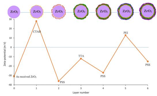
Fig. 5 Zeta-potential measurement of ZrO<sub>2</sub> nanoparticles and obtained compounds after each stage of the LBL process (reproduced from ref. 87 with permission from [Elsevier], copyright [2021])
