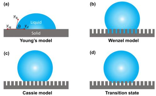
Fig. 7 Typical wetting behavior of a droplet on a solid surface. (a) Young's model, (b) Wenzel model, (c) Cassie model, and (d) transition state.
