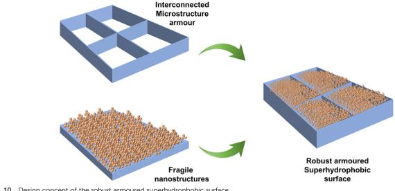
Fig. 10 Design concept of the robust armoured superhydrophobic surface.
