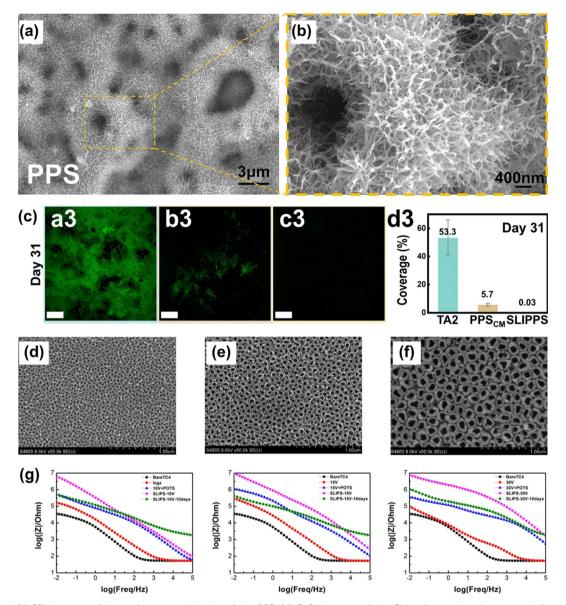
Fig. 17 (a) and (b) SEM images of the surface morphologies of the PPS. (c) CLSM images of the Chlorella covering (reproduced from ref. 198 with permission from [Elsevier], copyright [2023]). (d)-(f) FE-SEM images of the TC4 anodic films formed at different voltages (10 V, 15 V, and 30 V). (g) Electrochemical impedance spectra of samples immersed in 3.5 wt% NaCl solution for 10 days (reproduced from ref. 199 with permission from [American Chemical Society], copyright [2019]).
