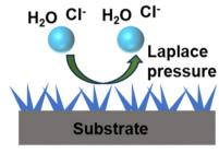
Schematic diagram of the anti-corrosion mechanism on SHSs.
