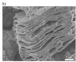
of an ML-MXene filtered and bucky paper sample. The bucky paper was carefully prepared, dried, and used as the sample for the measurement. The recorded electrical conductivity value yielded a noteworthy 1208 s cm<sup>-1</sup>.
