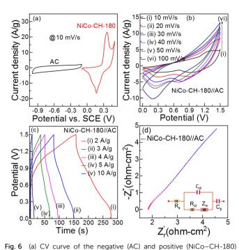
electrode at 10 mV s<sup>-1</sup> in a three-electrode set up. (b) CV curves for the ASC at various scan rates (10-100 mV s), (c) GCD curves at different current densities (2-10 A g<sup>-1</sup>), and (d) Nyquist plot of the NiCo-CH-180// AC ASC (two-electrode device)
