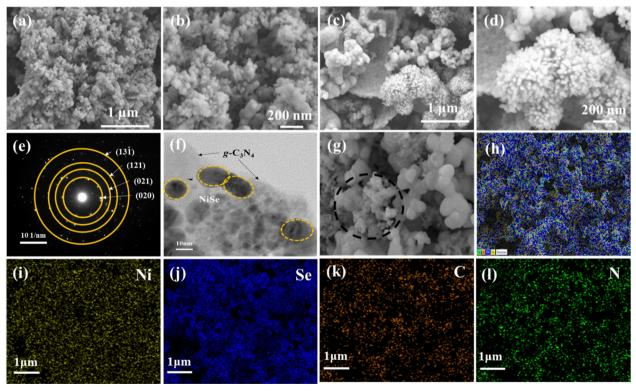
Fig. 2 FE-SEM images of (a), (b) NiSe<sub>2</sub>, (c), (d) NiSe<sub>2</sub>/g-C<sub>3</sub>N<sub>4</sub>, and (e), (f) HR-TEM of NiSe<sub>2</sub>/g-C<sub>3</sub>N<sub>4</sub>. (g)-(l) Energy dispersive spectroscopy (EDS) mapping of elements Ni, Se, C, and O in NiSe<sub>2</sub>/g-C<sub>3</sub>N<sub>4</sub>.
