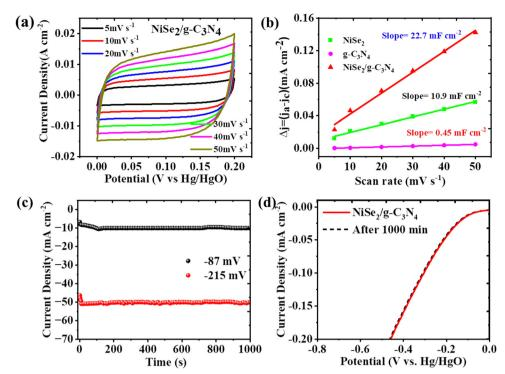
Fig. 5 (a) CV of NiSe<sub>2</sub>/g-C<sub>3</sub>N<sub>4</sub> at 5–50 mV s<sup>-1</sup> scan rates, (b) estimated values of  $C_{dl}$  for g-C<sub>3</sub>N<sub>4</sub>, NiSe<sub>2</sub>, and NiSe<sub>2</sub>/g-C<sub>3</sub>N<sub>4</sub>. (c) Chronoamperometric measurement at constant potentials -0.087 and 0.215 V vs. RHE for NiSe<sub>2</sub>/q-C<sub>3</sub>N<sub>4</sub>. (d) LSV curves of NiSe<sub>2</sub>/q-C<sub>3</sub>N<sub>4</sub> before and after 1000 min.
