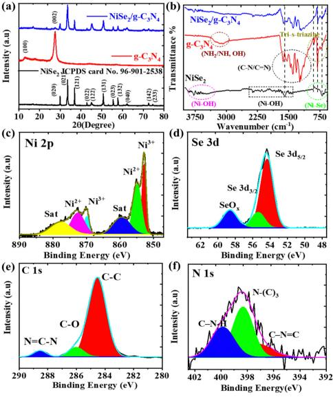
Fig. 1 (a) XRD and (b) FTIR patterns for the NiSe<sub>2</sub>,  $g-C_3N_4$ , and NiSe<sub>2</sub>/ $g-C_3N_4$  nanocomposite. (c) – (f) XPS patterns of Ni 2p, Se 3d, C 1s, and N 1s in NiSe<sub>2</sub>/ $g-C_3N_4$  nanocomposite. g-C<sub>3</sub>N<sub>4</sub> nanocomposite.
