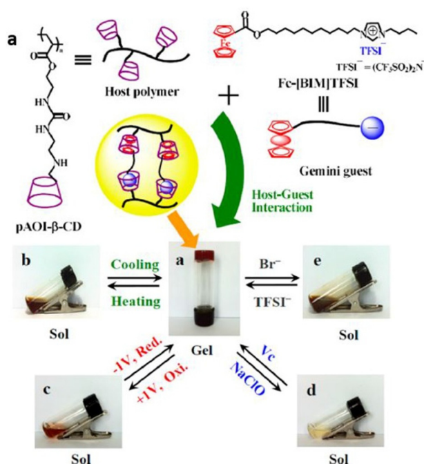
Fig. 46 (a) Preparation of ionic liquid gemini guest cross-linked electroactive supramolecular gels and (b–e) their assembly and disassembly induced by multistimuli. Reproduced from ref. 225 with permission from ACS, Copyright [2014].
