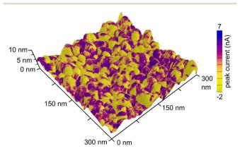
2 Three-dimensional image of the topography electrodeposited Pt coated with a 0.5 nm thick layer of Nb2O5. The topography is overlaid with an electrical conductivity map (e.g., peak current values) as measured by conductive atomic force microscopy (C-AFM)
