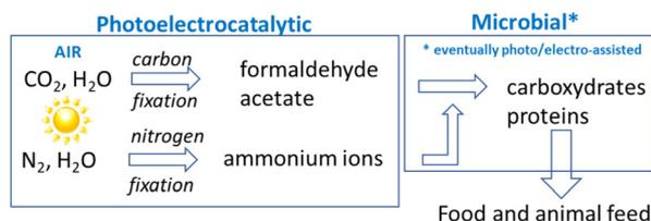
**Fig. 7** Producing sustainable food from the air in artificial-leaf devices.
