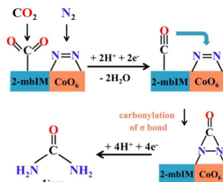
**Fig. 6** Reaction mechanism of urea electrocatalytic synthesis (at low potential) from CO<sub>2</sub> and N<sub>2</sub> on Co-PMDA-2mbIM. Adapted with permission by Yuan *et al.*<sup>155</sup> – ESI. Copyright RCS 2022.
