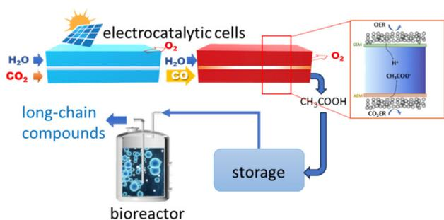
**Fig. 8** *In vitro* artificial sugar synthesis system. CO<sub>2</sub> was first converted to pure acetic acid through two-step electrolysis; this product was then directly fed for microorganism fermentation in a bioreactor to produce long-chain compounds, for example, glucose. In the inset: schematic illustration of CO reduction (COR) to pure acetic acid in the solid-electrolyte reactor. Original figure based on Zheng *et al.*<sup>181</sup> scheme.
