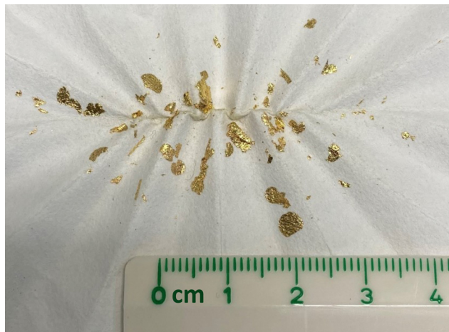
Fig. 6 Collected Au after filtration from filtrates.
