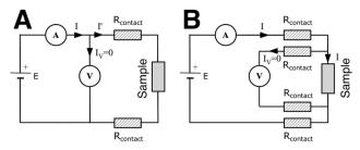
Fig. 10 Circuit diagrams of (A) two-point probe and (B) four-point probe method
