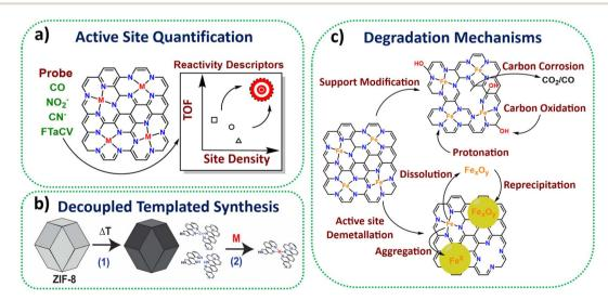
Fig. 1 Schemes representing some highlighted achievements in method development and understanding in the past 10 years for M-N-Cs. (a) Active site quantification. (b) Decoupled synthesis consisting of pyrolysis of active site template materials, followed by active metal loading. (c) Identified degradation mechanisms of Fe-N-C.
