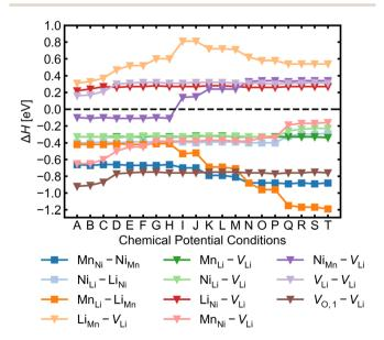
Fig. 6 Defect complex association energy  $\Delta H$  for a selection of stoichiometric complexes (denoted by squares) and non-stoichiometric complexes (denoted by triangles) calculated at the selfconsistent Fermi level over 20 different growth conditions from A (Orich, p-type) to T (O-poor, n-type).
