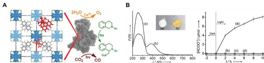
Fig. 8 (A) Schematic illustration of the MOF  $[\text{Re}^{\text{I}}(\text{CO})_3(\text{bpydc})\text{Cl}]$  for photocatalytic  $\text{CO}_2$  reduction.<sup>78</sup> Copyright 2011, American Chemical Society. (B) (left) UV/Vis spectra (a) MIL-125(Ti) and (b)  $\text{NH}_2$ -MIL-125(Ti) and the inset shows a photo of the samples of the corresponding samples and (right) the amount of  $\text{HCOO}^-$  produced as a function of the irradiation time.<sup>79</sup> Copyright 2012, Wiley.
