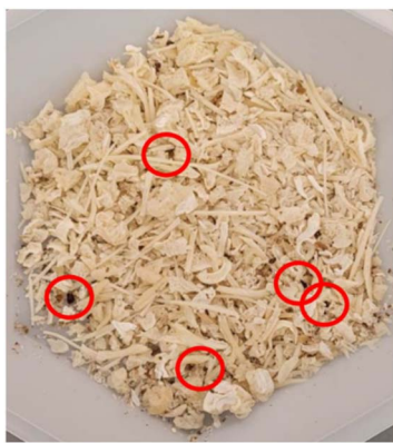
Fig. 5 Example of sHAP that would be considered a fail response (crude sHAP). Small and dark pieces of flesh remain within the sample (circled in red).
