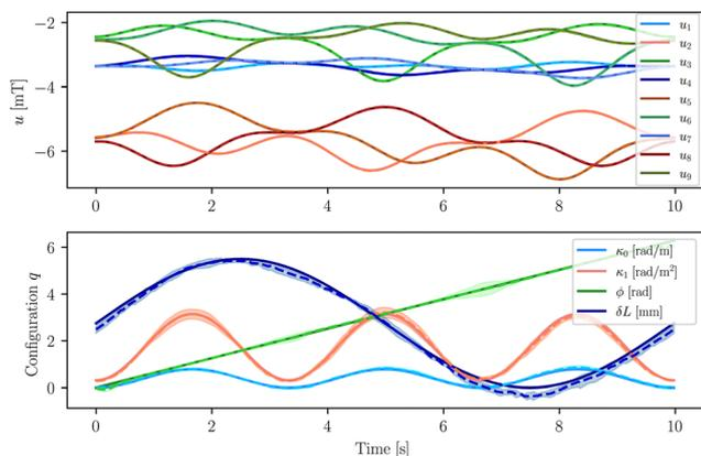
**Fig. 6** Sensor measurement predictions (top) and configuration estimates (bottom) for an affine curvature segment with nine magnetic sensors. We plot the ground-truth values  $u$  and  $q$  in solid, the estimate  $\hat{u}$  and  $\hat{q}$  as a mean over three random seeds with dashed lines and the standard deviation as an error band. The random seed determines at the start of the training the initialization of the neural network weights.
