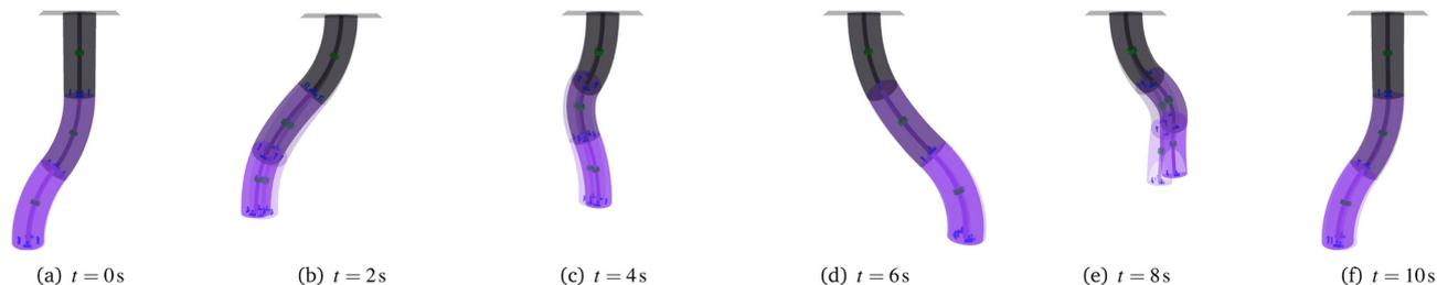
**Fig. 5** Sequence of stills for simulated sensor failure as shown in Fig. 4(b): the number of sensors per segment, which are rendered in blue, is reduced from four to three at  $t = 5$  s. We visualize the ground-truth shape of the soft robot with full opacity and the estimated configuration with slight transparency. The magnets are rendered in green and the three segments are visualized in a color sequence from black to violet.
