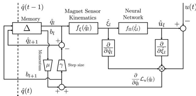
Fig. 3 A block-diagram of the gradient descent as an iterative update loop for the configuration belief  $\hat{q}(t)$ . The gradient descent is initialized with the optimized solution  $\hat{q}_0 = \hat{q}(t-1)$  from the previous time-step. Note that during the iterative loop,  $\hat{q}_{l+1}$  updates  $\hat{q}_l$  in the memory block.
