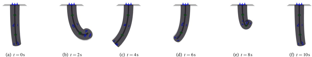
**Fig. 7** Sequence of stills for a simulated affine curvature robot. We visualize the ground-truth shape of the soft robot with full opacity and the estimated configuration with slight transparency. The two magnets are rendered in green and the nine sensors in blue.
