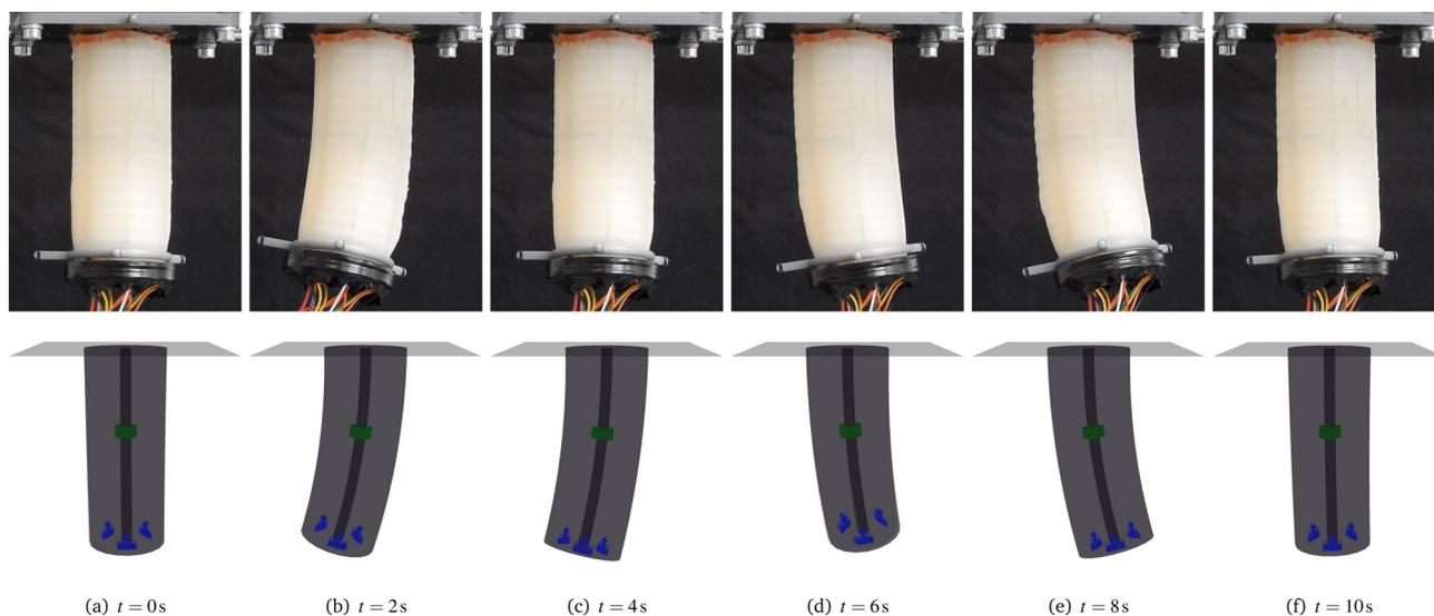
**Fig. 11** Sequence of stills for inference on T3 (full lemniscate) of a model trained on T5. The top row shows camera recordings of an external view and the sequence in the bottom row consists of renderings of the ground-truth state (in full opacity) and the estimated segment shape (slightly transparent). The sensors are colored in blue and the ring magnet integrated into the backbone is shown in green.
