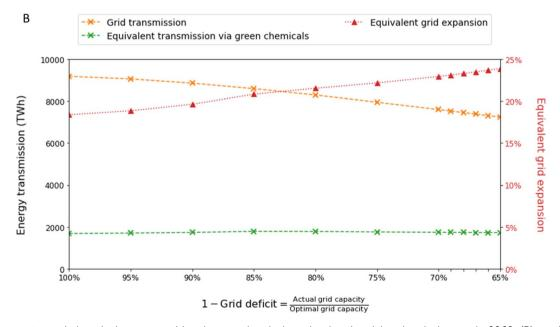
Fig. 8 (A) Energy transmission via the power grid and green chemicals under the electricity-chemical nexus in 2060; (B) sensitivity analysis assuming at most a 35% deficit in utilizable grid transmission capacity under the electricity-chemical nexus in 2060.
