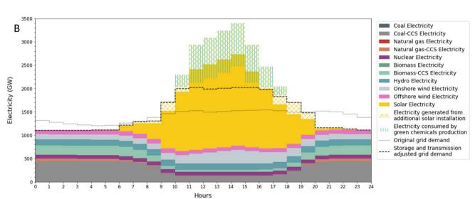
Fig. 5 (A) Capacity and annual operation of power generation technologies for different scenarios in 2060; (B) average day hourly dispatch of different technologies under the electricity-chemical nexus in 2060.
