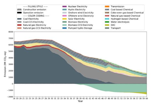
Fig. 3 GHG emission pathway of the electricity-chemical nexus in China towards carbon neutrality.
