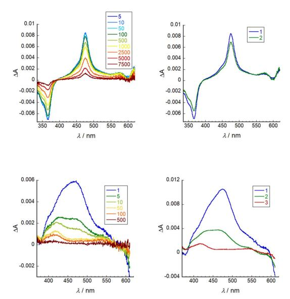
Fig. 6 Left: transient absorption spectra ( $\lambda_{ex} = 640$  nm) of SF5-3 in THF (top) and SF5-3|NiO (bottom). Right: evolution associated spectra of **SF5-3** in THF where 1 = 260 ps and 2 = 4.0 ns (top) and **SF5-3**|NiO where 1 = 0.87 ps, 2 = 8.3 ps, 3 = 230 ns (bottom).
