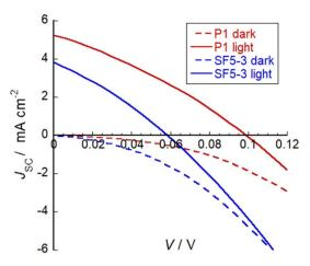
Fig. 7 Plot of current density against voltage for illuminated devices containing dye SF5-3 and the benchmark dye P1. Electrolyte composition: 0.1 M Lil and 1 M  $I_2$  in MeCN.
