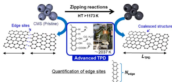
Fig. 1 Schematic of HT of CMS and the accompanied graphene-zipping reactions. The advanced temperature-programmed desorption (TPD) is used to quantify the carbon edge sites and calculate the average graphene-domain size ( L_{\text{TPD}} ).
