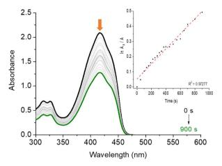
Fig. 5 DPBF photo-oxidation experiment in DMF solution by irradiation with red-light LED source (660 nm; irradiance of 100 mW cm $^{-2}$  and a total light dosage of 90 J cm $^{-2}$ ) in the presence of corrole  $H_3$ -LapCor. The inset shows the first order kinetic profile.
