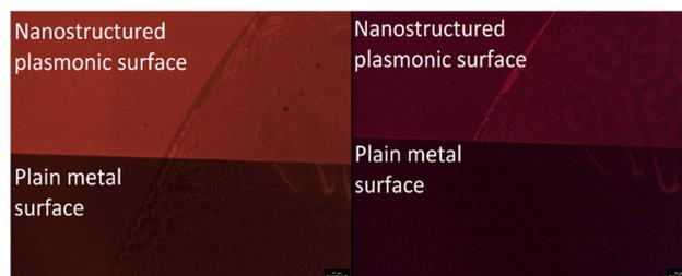
**Fig. 5** Fluorescence microscope images: (left)  $615 \text{ nm}$   $\text{Eu}^{3+}$  emission, and (right)  $660 \text{ nm}$  FRET emission, obtained for Eu-HQA + Alexa647 surfaces on nanostructured plasmonic surface (top) and on plain metal surface (bottom). The tilted lines in the images represent the left-side edge of the Alexa647 droplet.
