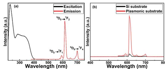
**Fig. 4** (a) Luminescence properties of Eu-HQA thin films: (a) excitation ( $\lambda_{\text{em}} = 615 \text{ nm}$ ) and emission ( $\lambda_{\text{ex}} = 250 \text{ nm}$ ) spectra for Eu-HQA thin film grown on silicon substrate; (b) 20-fold enhanced emission intensity for Eu-HQA thin film grown on a plasmonic substrate in comparison to silicon substrate ( $\lambda_{\text{ex}} = 400 \text{ nm}$ ).
