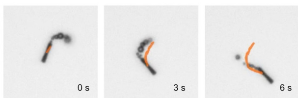
A Time lapse of MnO 2 micromotor trajectories at 2 wt. % H 2 O 2
