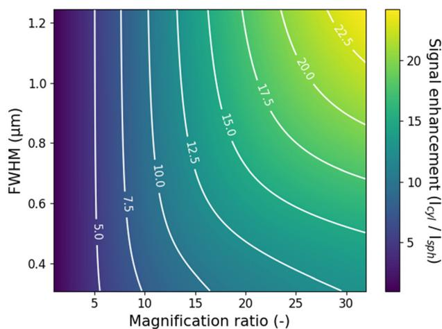
**Fig. 5** Simulations of the dependence of the signal enhancement ( $I_{\text{cyl}}/I_{\text{sph}}$ ) on the magnification ratio ( $M_y/M_x$ ) and the time-integrated FWHM of the energy carrier population for a detector size of  $20 \mu\text{m}$  and  $y$ -axis magnification of  $M_y \sim 400$ . A signal enhancement up to  $\sim 25$  is predicted for magnification ratios of 30 and FWHM of  $1.2 \mu\text{m}$ . A Voigt was chosen as population distribution.
