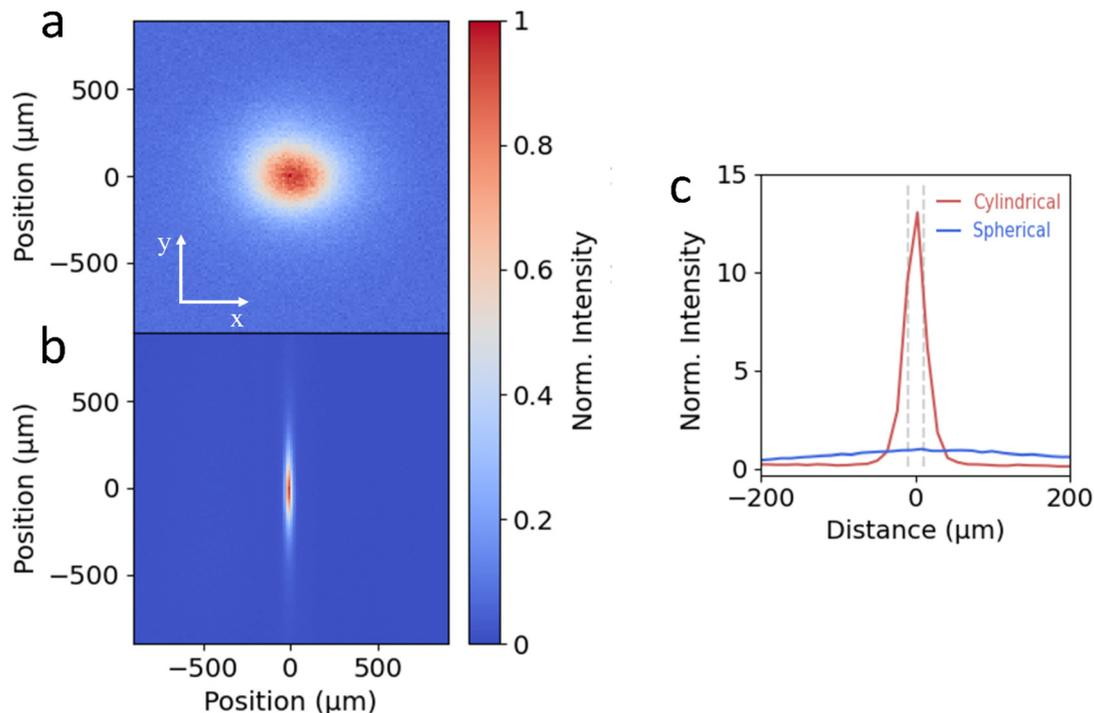
**Fig. 2** (a and b) Visualization of the projection of the emission intensity of the 2D perovskite with the spherical and the cylindrical lenses, respectively. (c) Intensity profiles along the  $x$ -axis of the center of the population for the cylindrical (red) and the spherical (blue) lenses. Dashed grey lines denote the APD size ( $20\ \mu\text{m}$ ). Intensities in c are normalized to the maximum intensity detected with the spherical lens.
