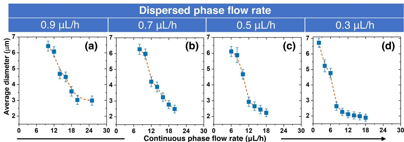
Fig. 4 Relationship between QD-MB diameter and continuous flow rates. The dispersed flow rate was set at 0.9  $\mu\text{L h}^{-1}$  (a), 0.7  $\mu\text{L h}^{-1}$  (b), 0.5  $\mu\text{L h}^{-1}$  (c), and 0.3  $\mu\text{L h}^{-1}$  (d). Increasing the continuous flow rate led to a decrease in the average diameter of QD-MBs. The coefficient of variance for the size distribution was less than 10%.
