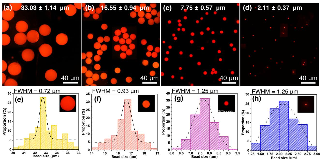
Fig. 2 Fluorescence micrographs and size distribution of QD-MBs of different sizes, depending on the flow rate. (a–d) Micrographs of QD-MBs with average diameters of 33.03  $\mu\text{m}$ , 16.55  $\mu\text{m}$ , 7.75  $\mu\text{m}$ , and 2.11  $\mu\text{m}$ , respectively. (e–h) Corresponding size distribution histograms of the QD-MBs.
