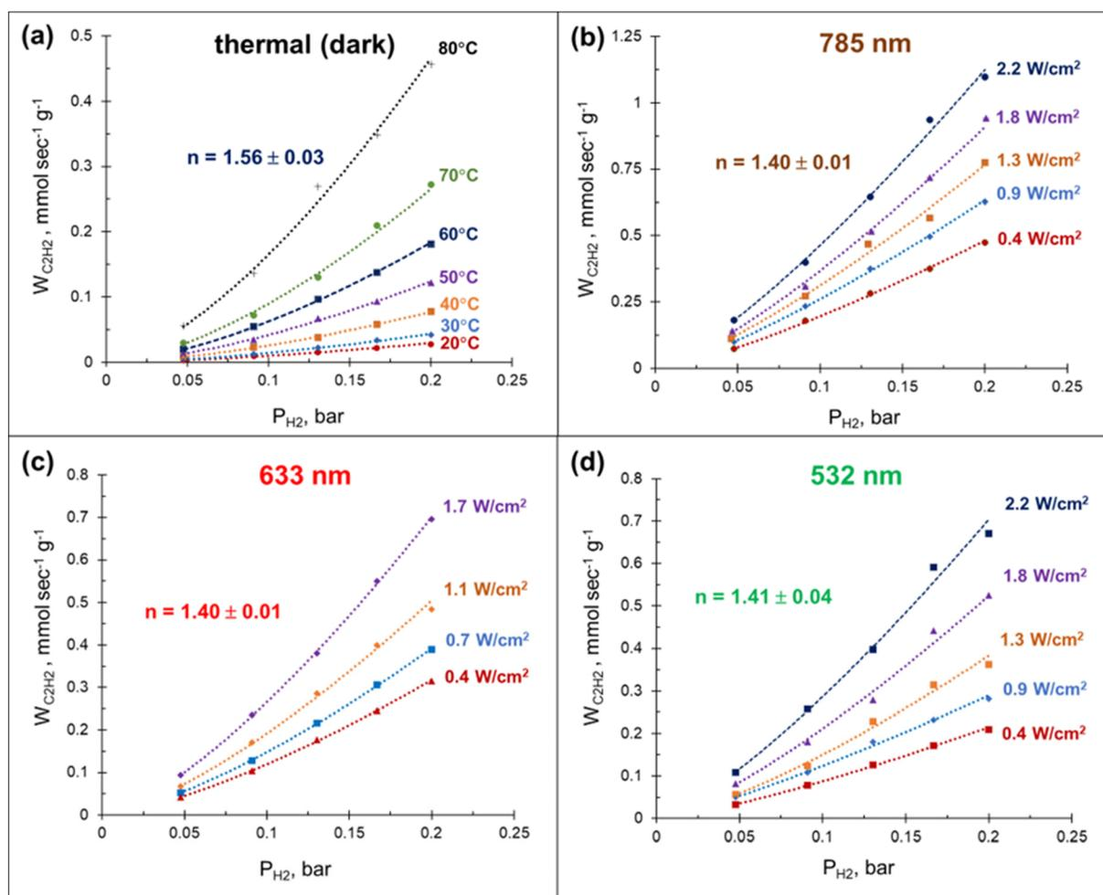
Fig. 4 Acetylene conversion rate over 3%Pd–Mg/GS as a function of hydrogen partial pressure  $P_{\text{H}_2}$ . (a) Thermal (dark) and photo mediated with laser light illumination wavelengths of (b) 785 nm, (c) 633 nm, and (d) 532 nm. The  $P_{\text{C}_2\text{H}_2}$  was kept constant at 0.05 bar and the reaction order ( $n$ ) reported is with respect to  $\text{H}_2$ .
