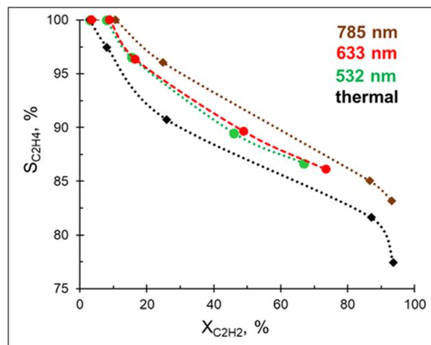
**Fig. 3** Steady-state ethylene selectivity as a function of acetylene conversion over 3%Pd–Mg/GS under thermal and photo-mediated activation. The catalyst surface temperature was maintained at 60 °C for both thermal and photocatalytic experiments and the H<sub>2</sub>:C<sub>2</sub>H<sub>2</sub> was fixed at 3 : 1.
