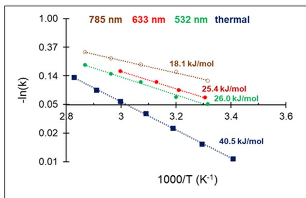
Fig. 5 Arrhenius plot of C<sub>2</sub>H<sub>2</sub> hydrogenation and apparent activation energies for photo- and thermocatalytic experiments over 3%Pd–Mg/GS.
