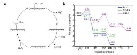
Fig. 3 (a) Schematic diagram of the H<sub>2</sub>O<sub>2</sub> decomposition reaction cycle on Cu @MoS<sub>2</sub>-Vs. (b) Energy profiles of Cu@MoS<sub>2</sub>-Vs in neutral, acidic and alkaline conditions. The numbers represent the energy (eV) at each state. The abscissa TS, M, and P represent transition states, intermediates and products, respectively.
