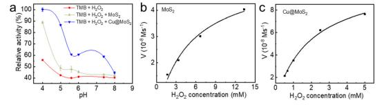
Fig. 5 (a) Relative catalytic activity of the MoS<sub>2</sub> and Cu@MoS<sub>2</sub> as peroxidase mimics under different pH values at 37 °C tested by UV-vis absorption of oxTMB. The velocity of the reaction between 'OH and the various concentrations of H<sub>2</sub>O<sub>2</sub> in the presence of (b) MoS<sub>2</sub> and (c) Cu@MoS<sub>2</sub>. The successful Cu loading on the MoS<sub>2</sub> surface was well in agreement with the DFT calculations.
