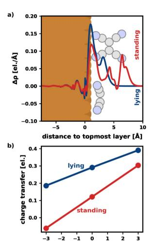
Fig. 3 Visualization of the charge transfer. (a) Plane-averaged electron density difference between a field  $F=3~{\rm V~mm^{-1}}$  and 0 V nm $^{-1}$  for the most stable lying/standing adsorption geometries. The spatial extent of adsorption geometries of a lying and a standing molecule are indicated. (b) Net charge transfer into the molecule (calculated *via* Mulliken analysis) for the most stable lying/standing adsorption geometry.
