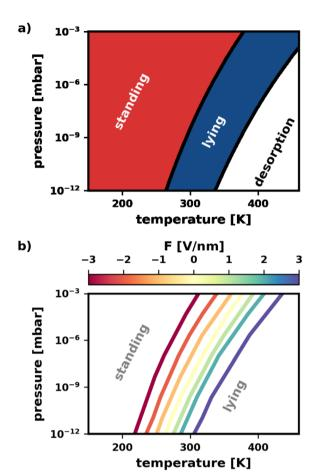
Fig. 6 Phase diagram showing the relationship between most stable polymorph category and pressure, temperature, and electric field. Pressure refers to the partial pressure of the TCNE in gas phase. (a) Pressure–temperature phase diagram for  $F = 0 \text{ V nm}^{-1}$  (i.e., no field applied). The red phase corresponds to standing polymorphs, the blue phase to lying polymorphs. (b) Change of the pressure-temperature phase boundary between standing and lying for different electric
