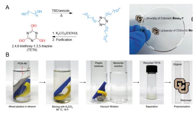
Fig. 14 (A) Depolymerization and synthesis of polycyanurate network polymers. (B) Polycyanurates can be depolymerized in the presence of ethanol and  $K_2CO_3$  added as a catalyst. Reproduced in part with permission from ref. 40. Copyright 2022 *Nature Chem*.
