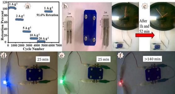
Fig. 16 Investigation of practical applications. (a) Long-term cycling stability of the AC//Ni/CoMOF-rGO device at different current densities. Practical applications of the AC//Ni/Co-MOF-rGO device: (b) a simple laboratory prototype of the fabricated device; (c) turning on a clock for 1 h and 52 min; sequential lighting up of (d) blue, (e) green, and (f) red LEDs for a definite time. Reproduced from ref. 170 with permission from Elsevier Ltd, Copyright 2018.
