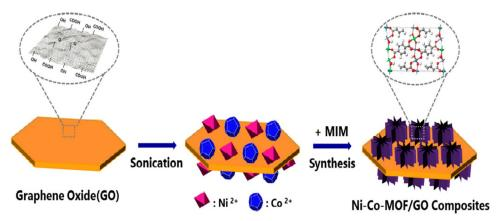
Fig. 15 The scheme for the preparation process of Ni-Co-MOF/graphene oxide composites. Reproduced from ref. 168 with permission from Elsevier Ltd, Copyright 2019.
