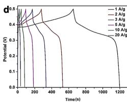
Fig. 8 (a) CV curves of Ni-BTC and Ni-BTC@GO composites at 2 mV s $^{-1}$ , (b) GCD curves of Ni-BTC and Ni-BTC@GO composites at 1 A g $^{-1}$ , (c) CV curves of Ni-BTC@GO 2 at 2 $^{-1}$ 0 mV s $^{-1}$ , and (d) GCD curves of Ni-BTC@GO 2 at 1 $^{-2}$ 0 A g $^{-1}$ 1. Reproduced from ref. 151 with permission from American Chemical Society, Copyright 2023.
