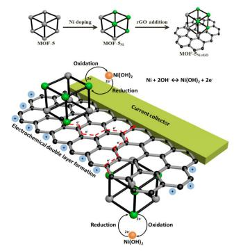
Scheme 3 The concept for Ni doping and incorporating rGO to form a composite of rGO and Ni-doped MOF-5 and its use as an electrode material that harnesses both the electrochemical double layer performance of rGO and the reversible redox reactions of Ni metal centres with a synergy that facilitates effective and efficient charge transfer processes. Reproduced from ref. 165 with permission from American Chemical Society, Copyright 2015.
