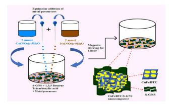
Scheme 4 Schematic illustration of the synthesis procedure of CuFeBTC/ S-GNS nanocomposite. Reproduced from ref. 175 with permission from Elsevier Ltd, Copyright 2019
