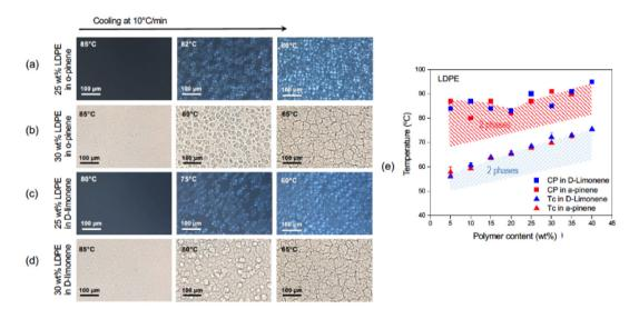
Fig. 3 (a and c) Polarized and (b, d) non-polarized optical microscopy cloud point (CP) measurements; (e) corresponding phase diagram obtained by cloud point and DSC crystallization ( $T_c$ ) measurements for LDPE in α-pinene and p-limonene.
