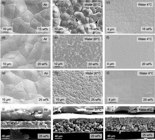
Fig. 4 Surface morphology of pure PP membranes prepared with 15 wt% (a-c), 20 wt% (d-f), and 25 wt% (g-i) PP solutions in α-pinene and quenched in air at room temperature (a, d and q), water at 20 °C (b, e and h), and water at 4 °C (c, f and i); cross-section images of membranes prepared from 25 wt% PP solutions in  $\alpha$ -pinene quenched under different conditions (j-l).
