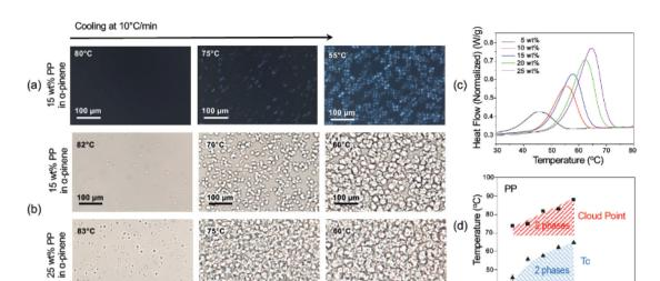
Fig. 2 (a) Polarized and (b) non-polarized optical microscopy cloud point (CP) measurements; (c) crystallization ( $T_c$ ) measurement by DSC temperatures for PP in α-pinene; and (d) corresponding phase diagram.
