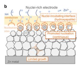
Fig. 1 Comparison between the conventional and nuclei-rich Zn plating strategy. Schematic of Zn plating on (a) conventional and (b) nuclei-rich Zn electrodes
