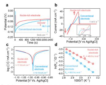
**Fig. 4** Enhanced Zn plating and stripping kinetics. (a) Galvanostatic voltage profiles, (b) cyclic voltammograms curves, (c) Tafel plots, and (d) Arrhenius plots of Zn plating and stripping on conventional and nuclei-rich electrodes.
