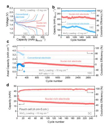
**Fig. 6** High capacity and high stability  $Zn-MnO_2$  full cells enabled by the nuclei-rich anode. (a) Voltage profile of  $Zn-MnO_2$  full cells with conventional and nuclei-rich Zn electrodes. The long-term-cycling profile of  $Zn-MnO_2$  full cells under different conditions: (b)  $MnO_2$  loading at 2 mg cm $^{-2}$ , (c)  $MnO_2$  loading at 10 mg cm $^{-2}$ , and Zn foil thickness at 0.01 mm (N/P ratio = 1.9), and (d)  $MnO_2$  loading at 10 mg cm $^{-2}$  in pouch cells (single layer).
