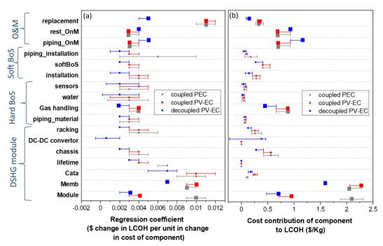
Fig. 3 (a) Estimated regression coefficients for each component considered in DHSG system (b) cost contribution of component to LCOH in \$ per kg assuming baseline LCOH and component cost. Components that have the biggest impact on the LCOH are highlighted with larger markers.
