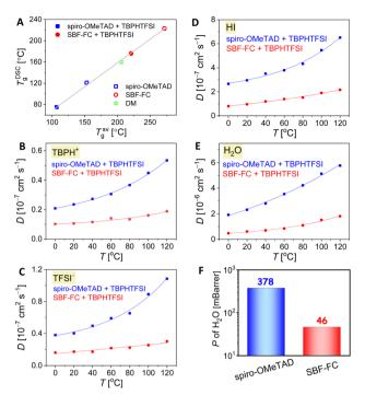
Fig. 4 (A) Correlation between theoretical and experimental glass transition temperatures. (B-E) Plots of the diffusion coefficient (D) of species in the 15 wt% TBPHTFSI containing composites as a function of temperature (7): (B) TBPH cation; (C) TFSI anion; (D) HI; and (E) H2O. (F) Theoretical permeability (P) of H<sub>2</sub>O in the composites at room temperature.
