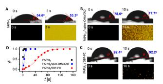
Fig. 5 (A–C) Temporal evolutions of the water contact angle ( $\theta$ ) and the polarized optical microscopy (POM) image upon dripping a water droplet on three samples: (A) FAPbI<sub>3</sub>, (B) spiro-OMeTAD covered FAPbI<sub>3</sub>, and (C) SBF-FC covered FAPbl3. The size of the POM image is 500  $\mu m$   $\times$ 250 μm. In the yellow region, perovskite is decomposed. (D) Plots of the yellow region percentage  $(\phi)$  as a function of time (t).
