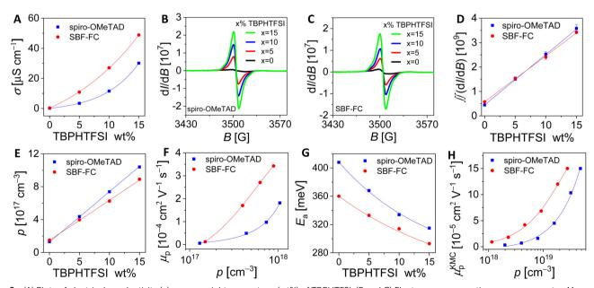
Fig. 2 (A) Plots of electrical conductivity ( $\sigma$ ) versus weight percentage (wt%) of TBPHTFSI. (B and C) Electron paramagnetic resonance spectra. Magnetic field strength, B; first derivative of absorption intensity, dI/dB. (D) Quadratic integral of dI/dB. (E) Hole density (p). (F) Plots of hole mobility ( $\mu_p$ ) versus p. (G) Activation energy ( $E_a$ ). (H) Kinetic Monte Carlo simulated hole mobility ( $\mu_p^{KMC}$ ).
