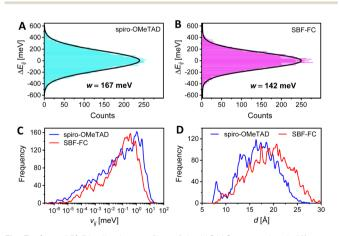
Fig. 3 (A and B) Distribution profiles of the HOMO energy level difference  $(\Delta E_{ii})$ . The black solid lines refer to the Gaussian fits to acquire the energetic disorders, being 167 meV for spiro-OMeTAD and 142 meV for SBF-FC. (C and D) Profile of transfer integral  $(v_{ij})$  and centroid distance (d).
