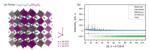
Fig. 1 Crystal structure of CCTM2112. (a) SCAN+U-optimized SQS for Pnma CCTM2112, where Ca, Ce, Ti, Mn, and O are blue, green, gray, purple, and red, respectively, and the polyhedra depict the B-site cations. Lattice constants (a, b, and c) are color-coded according to the axis labels. (b) Rietveld refinement of the as-synthesized CCTM powder. The green and orange tick marks, show the locations of CCTM and CeO2 reflections, respectively.
