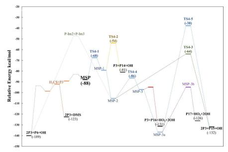
Fig. 14 Relative energy diagram for decomposition of the MSP intermediate formed in the AMS oxidation initiated by OH radicals in the absence of NO<sub>x</sub> at the M06-2X/GD3/aug-cc-pVTZ level.
