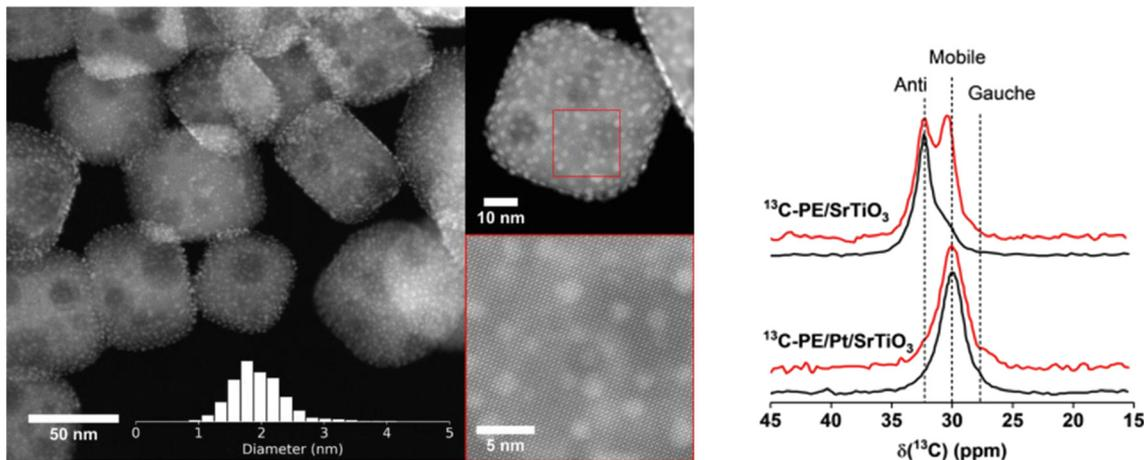
Fig. 3 STEM images of Pt/SrTiO<sub>3</sub> catalyst (left). <sup>13</sup>C MAS (red) and CPMAS (black) spectra of <sup>13</sup>C-enriched PE adsorbed on the SrTiO<sub>3</sub> support (top), and Pt/SrTiO<sub>3</sub> catalyst (right). Reproduced from ref. 47 with permission from American Chemical Society.
