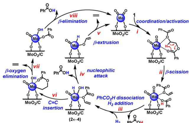
Fig. 10 The mechanism for the hydrogenolysis of PET over the C/MoO<sub>2</sub> catalyst. Reproduced from ref. 82 with permission from Wiley.
