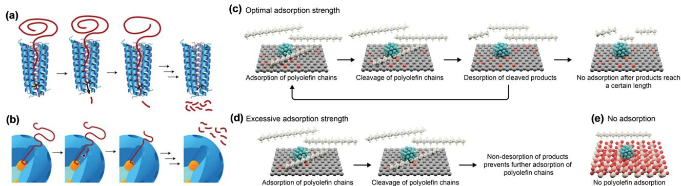
Fig. 4 Processive deconstruction of macromolecules (a) over enzymes and (b)  $m\text{SiO}_2/\text{Pt}/\text{SiO}_2$  catalyst. Adsorption/desorption processes on various carbon supports (c–e). Reproduced from ref. 42 and ref. 40 with permission from Springer Nature and Wiley, respectively.
