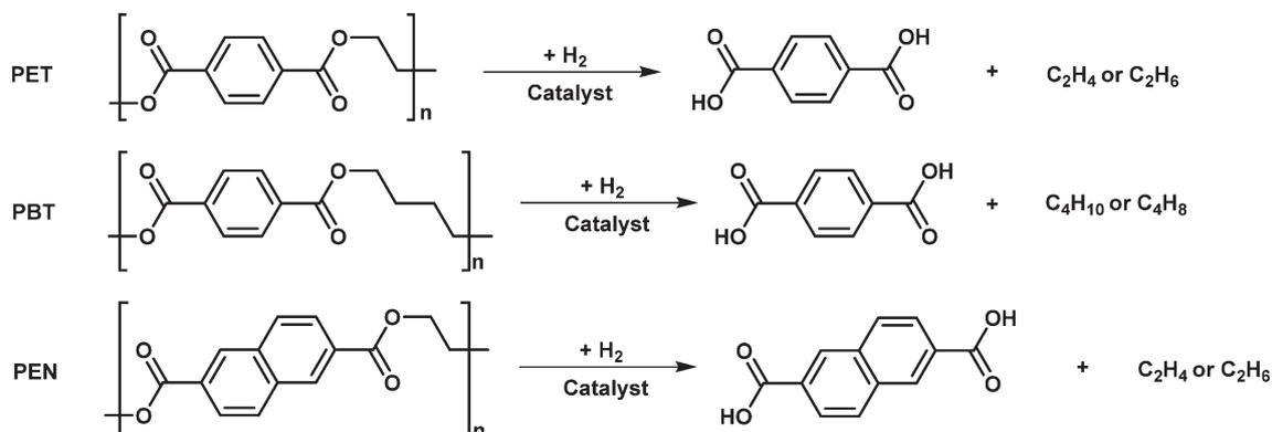
Fig. 9 Hydrogenolysis of PET, PBT and PEN.
