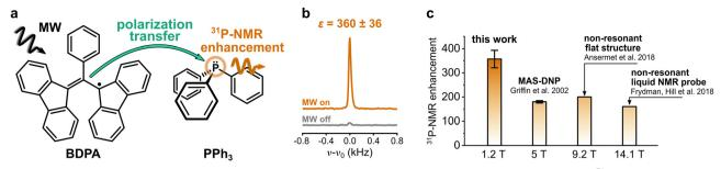
Fig. 1 (a) Sketch of the polarization transfer process between the PA (BDPA radical) and the target molecule (PPh<sub>3</sub>). (b) <sup>31</sup>P-NMR spectra of PPh<sub>3</sub> in benzene doped with BDPA recorded at 1.2 T with and without MW irradiation. (c) 31P-NMR enhancements reported at different magnetic fields for PPh<sub>3</sub> in benzene (fluorobenzene at 9.2 T) doped with BDPA radical.
