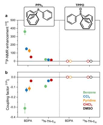
Fig. 2 (a)  $^{31}\text{P-NMR}$  enhancements recorded at 1.2 T and (b) coupling factors calculated with egn (1) for both PPh<sub>3</sub> and TPPO doped with BPDA and 15N-TN-d<sub>16</sub> in different solvents.
