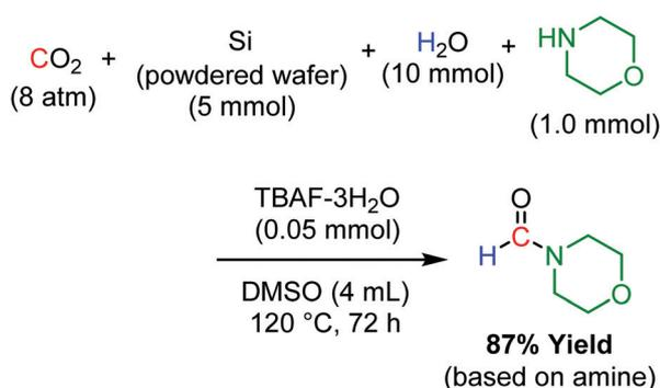
Scheme 3 Reductive functionalisation of CO<sub>2</sub> with an amine.
