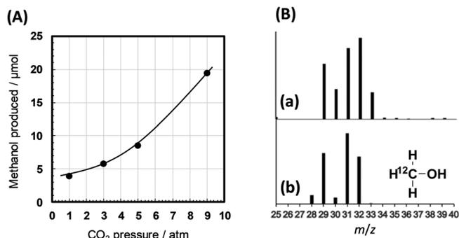
Fig. 6 (A) Effect of CO<sub>2</sub> pressure on the methanol yield. Reaction conditions: powdered silicon wafer (5 mmol; diameter < 20 μm), CO<sub>2</sub>, H<sub>2</sub>O (10 mmol), TBAF-3H<sub>2</sub>O (0.85 mmol), DMSO (2 mL), 95 °C, 24 h. Yield was determined by GC-FID using an internal standard technique. (B) Mass spectra of methanol produced in the reactions using (a) <sup>13</sup>CO<sub>2</sub> and (b) <sup>12</sup>CO<sub>2</sub>.
