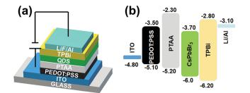
Fig. 6 (a) A schematic illustration and (b) flat-band energy level diagram of the CsPbBrz QLED device.
