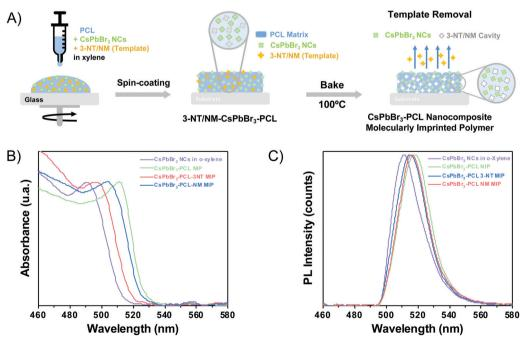
Fig. 1 (A) Schematic steps of the fabrication of the CsPbBr<sub>3</sub>-PCL 3-NT or NM MIP sensor. (B) UV-vis absorbance spectra and (C) emission spectra of CsPbBr<sub>3</sub> NCs in o-xylene (purple line) and embedded in the PCL polymer matrix without (green line), with 3-NT (blue line) and NM (red line) template.
