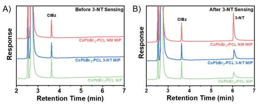
Fig. 6 Gas chromatograms of the CsPbBr<sub>3</sub>–PCL NIP and CsPbBr<sub>3</sub>–PCL 3-NT and NM MIP sensors (A) before and (B) after exposure to 3-NT vapours for 180 s
