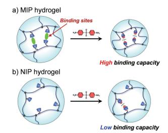
**Fig. 6** Schematic illustration of the dapsone adsorption into the MIP and NIP hydrogels.
