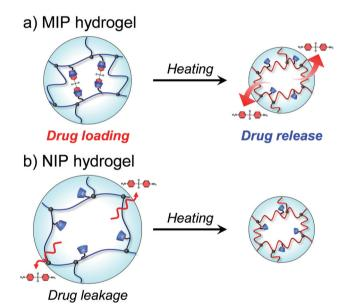
$\begin{tabular}{ll} Fig.~11 & Schematic illustration of drug release from MIP and NIP hydrogels with increasing temperature. \end{tabular}$
