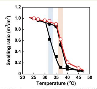
Fig. 4 Effect of temperature on the swelling ratio of the MIP (○), NIP (●) and PNIPAAm (■) hydrogels in water. Blue and red bars indicate the transition temperature of PNIPAAm and MIP & NIP hydrogels, respectively.
