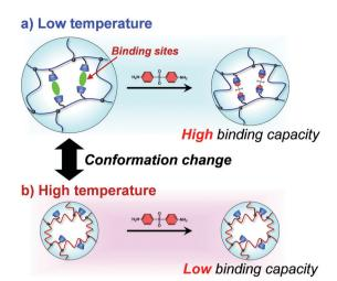
Fig. 1 Schematic illustration of the regulation of the drug-binding capacity by a conformational change of a thermoresponsive MIP hydrogel with dynamic molecular binding sites at low (a) and high (b) temperatures.
