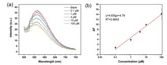
Fig. 6 (a) Fluorescence emission spectra of MIP particle suspension (0.5 mg mL<sup>-1</sup>) mixed with Cu<sup>2+</sup> solution at different concentrations in phosphate buffer (pH 8.5). (b) Linear relationship between the fluorescence intensity change and the logarithm of the Cu<sup>2+</sup> concentration.
