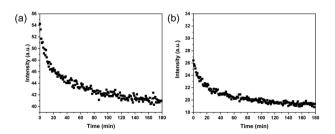
Fig. 4 (a) Change in fluorescence intensity of ARS-loaded MIP particles (0.5 mg mL $^{-1}$ ) measured after the addition of 1 M fructose. (b) Change in fluorescence intensity of ARS-loaded NIP particles (0.5 mg mL $^{-1}$ ) measured after the addition of 1 M fructose. The fluorescence intensity was measured at 560 nm in 20 mM phosphate buffer.
