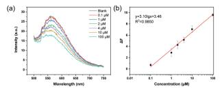
Fig. 7 (a) Fluorescence emission spectra of ARS-loaded MIP particles (0.5 mg mL $^{-1}$ ) mixed with Cu $^{2+}$  solution at different concentrations in phosphate buffer (20 mM, pH 8.5). (b) Linear relationship between the fluorescence intensity change and the logarithm of the Cu $^{2+}$  concentration.
