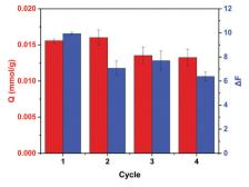
Fig. 8 Recycling and reuse of MIP nanoparticles for the adsorption of ARS and the detection of  $Cu^{2+}$  in buffer. Particle concentration: 0.5 mg mL $^{-1}$ ; ARS concentration: 0.02 mM. Cycle 1 used the original MIP particles, and cycles 2–4 used MIP particles regenerated from the previous cycle followed by reloading with 1 mM ARS and washing.
