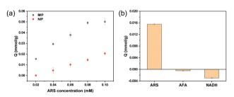
Fig. 2 (a) ARS binding on MIP and NIP particles measured in 20 mM phosphate buffer (pH 8.5). Concentration of MIP particles: 0.5 mg mL<sup>-1</sup>; incubation time: 1 h. (b) Binding of ARS, AFA and NADH on MIP particles measured in 20 mM phosphate buffer (pH 8.5). Initial concentration of the test compounds: 0.02 mM; concentration of MIP particles: 0.5 mg mL<sup>-1</sup>.
