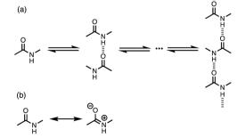
Fig. 1 (a) Supramolecular polymerisation of secondary amides. (b) Neutral and zwitterionic amide resonance structures.
