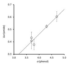
Fig. 8 Relationship between the H-bond donor properties of 4-X-phenols,  $\alpha$ (phenol), and the change in H-bond donor properties of the amide group in compounds 1–5 due to the intramolecular H-bond,  $\Delta\alpha$ (amide). The best fit line is y=0.20x-0.34.
