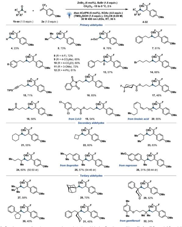
Scheme 2 Reaction scope of α-primary, -secondary and -tertiary aldehydes. Reaction conditions: 1b-1ae (0.3 mmol, 1.5 equiv.), benzoyl bromide (0.3 mmol, 1.5 equiv.), ZnBr<sub>2</sub> (0.01 mmol, 5 mol%), CH<sub>2</sub>Cl<sub>2</sub> (1 M), -15 to 0 °C, 2 h, then 2a (0.2 mmol, 1.0 equiv.), 4CzIPN (0.01 mmol, 5 mol%), KOAc (0.8 mmol, 4.0 equiv.), (TMS)<sub>3</sub>SiOH (0.3 mmol, 1.5 equiv.), MeCN (0.05 M), 30 W 450 nm LEDs, RT, 36 h. For experimental details, see the ESI.†
