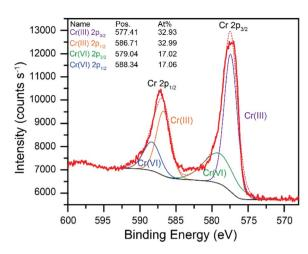
Fig. 5 XPS high-resolution core level data in the Cr 2p region (red, bold), along with the analysis: modeled background contribution (black), and contribution from both Cr(III) and Cr(VI), each with the expected contribution to the  $2p_{1/2}$  and  $2p_{3/2}$ . The dashed red trace represents the sum of all contributions from the analysis.
