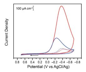
Fig. 1 Cyclic voltammogram (CV) on 3 mm diameter glassy carbon electrodes of a 0.20 mM (dashed lines) and 7.00 mM (solid lines)  $\rm K_2CrO_4$  solution in 0.10 M malate (red) and succinate (blue) buffers at pH 4.75. The cyclic voltammograms were collected at 0.10 V s<sup>-1</sup> in 1.00 M KCl supporting electrolyte.
