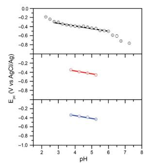
Fig. 3 Reduction peak potential values plotted as a function of pH for 0.20 mM Cr(vi) added as  $K_2CrO_4$  in 0.10 M citrate (black, top), malate (red, middle), and succinate (blue, bottom) buffers. Data collected in 1.00 M KCl electrolyte at scan rates of 0.10 V s<sup>-1</sup>. Citrate data from ref. 21. Slopes of 62.9 mV per pH ( $r^2 = 0.984$ ) and 62.4 mV per pH ( $r^2 = 0.991$ ) observed for malate and succinate respectively.
