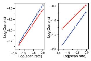
Fig. 2 Log of the absolute values of the reduction peak currents (mA) plotted as a function of the log of the scan rate (V s $^{-1}$ ) for cyclic voltammetry studies of 0.20 (left) and 7.00 mM (right)  $\rm K_2CrO_4$  added to 0.10 M malate (red) and succinate (blue) buffers at pH 4.75. Data in Fig. S1 and S2† Linear fit parameters summarized in Table 1.
