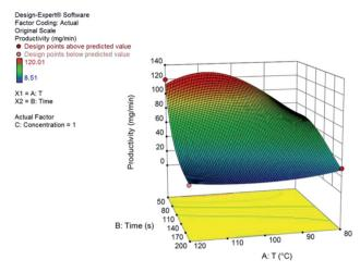
Fig. 3 Response surface for the productivity, in mg min<sup>-1</sup>, of furfuryl alcohol from furfural at 1.0 M. Coded variables are A for temperature and B for residence time.
