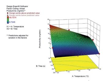
Fig. 7 Response surface for the productivity, in mg min<sup>-1</sup>, of DHMF from HMF.
