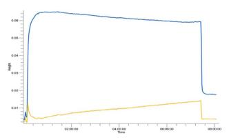
Fig. 6 Trend analysis of furfural reduction for the scale-up reduction. Wavenumbers selected:  $1713 \text{ cm}^{-1}$  (blue) to acetone and  $1680 \text{ cm}^{-1}$  (yellow) for the aldehyde. Reaction conditions: a 0.25 M solution of furfural in iso-propanol was pumped through a BZC column at  $120 \,^{\circ}\text{C}$  and 50 s residence time for 5.5 hours.
