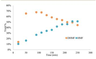
Fig. 8 Results of the scale-up reduction of HMF, with major decrease in catalytic activity. Reaction conditions: A 0.25 M solution of HMF in iso-propanol was pumped through a BZC column at 120  $^{\circ}$ C and 50 s residence time for 5.5 hours.
