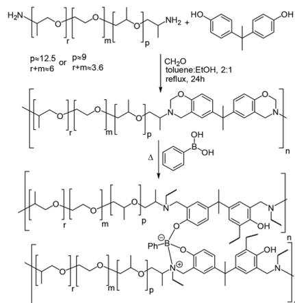
**Scheme 1** Synthesis of PPO<sub>900</sub>-Bz and PPO<sub>600</sub>-Bz and their simultaneous curing and reactions with PhB(OH)<sub>2</sub>.
