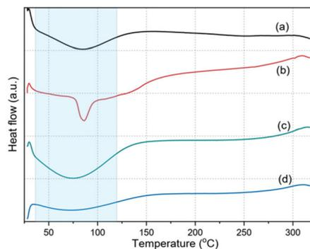
**Fig. 5** DSC thermograms (endotherm down) of the cured PPO<sub>900</sub>-Bz-Bor (a), and the 1<sup>st</sup> (b), 3<sup>rd</sup> (c) and 5<sup>th</sup> (d) cycles of the cured PPO<sub>900</sub>-Bz-Bor.
