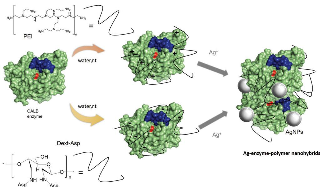
Fig. 3 Preparation of Ag-nanobiohybrids using enzyme-polymer conjugates.
